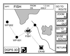
Figure 8-6 Plotter display, route selected as destination
